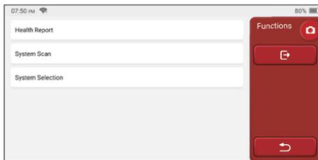
A. Health Report: this mode is to quickly check the vehicle and display the vehicle health report (it's available only when the the diagnosis software support this function). After clicking "quick test", the system starts scanning DTC respectively and show the result.
